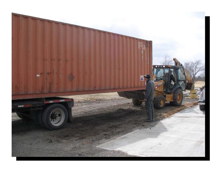
Lower the back end of the container to the ground assuring the container is resting on a pipe as shown below and not on the trailer.
