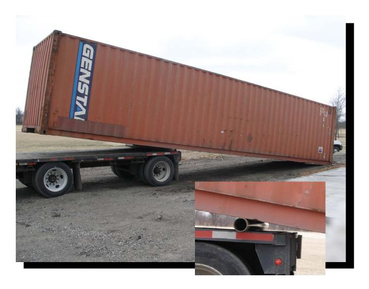
Chain and lift the front end of the container as shown and drive the trailer away from underneath the container.
