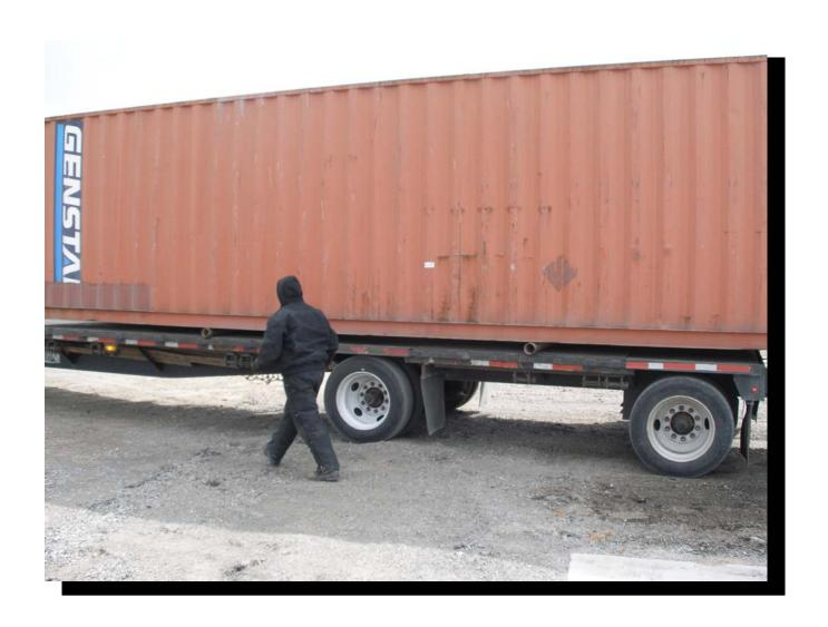
Roll the container off the trailer until it is just over half way off. Adjust the pipes as necessary throughout this process.
